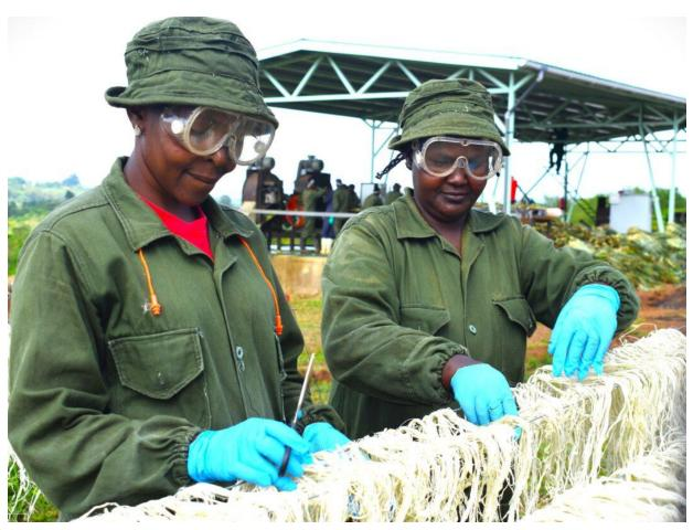
From Left, Lilian Ndungu and Agnes Kiloko arranging processed fibre to sun dry before going back to the machine for fine processing
